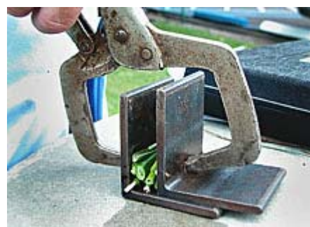
Fig. 3. Rice sap is extracted from basal stems using a sap press.
