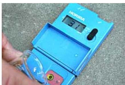
Fig. 4. Rice sap is poured onto a Cardy meter sensor for K^+ determination.
